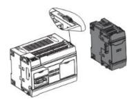
步骤 2. 将扩展模块对准主机接口推入到位后,反向推回锁扣进行扩展模块锁定。Then push the extension module into place against the mainframe interface and reverse the latch to lock the extension module.
