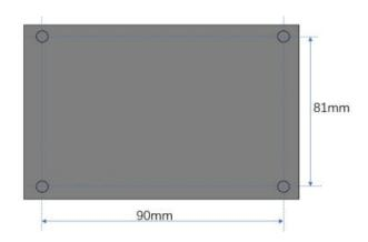
● 下图为具有 40 点 I/O 的 CPU 本体的安装孔间距 The following diagram shows the mounting holes for the 40 points I/O CPU.
