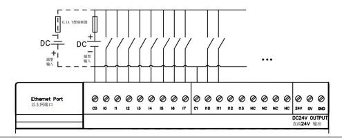
◆ 因为公共端 C0/C1/C2 彼此独立,使用相同输入类型时,请使用短接线将公共端连接。As the common terminals C0/C1/C2 are independent of each other, when using the same type of input, please connect the common terminals using short wires.
